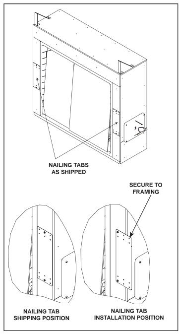
Figure 4.1 Positioning and Securing Nailing Tab
